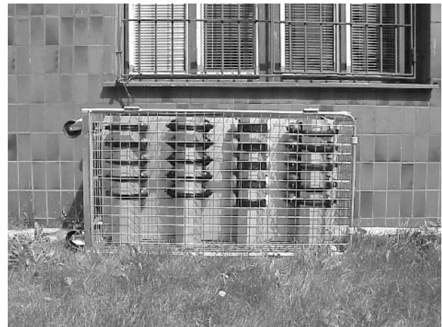
Fig. 1. Ear-muffs exposed to natural atmospheric conditions.
